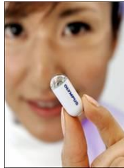
Camera pill with camera, transmitter and computer
