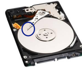
Hard disk read/write head (©Western Digital)
